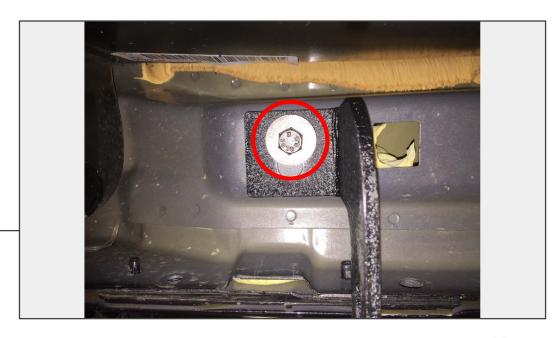
Position the new Rocker Step to the vehicle rocker panel bolt holes, and secure using the (3) M8x35mm bolts, lock washers, and flat washers through the rocker mount brackets.
