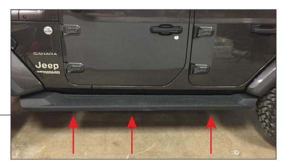
Begin by locating the (3) pinch weld mounting locations under the vehicle.
