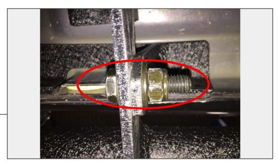
Connect the pinch weld brackets to the Rocker Step brackets by using (3) M10x35mm bolts, flat washers, and lock nuts. Then, fully tighten the rocker mount brackets from Step 5.
