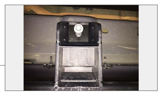
From under the vehicle, locate and remove each of the 13mm rocker panel mount bracket bolts.
