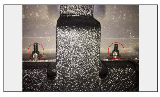
Align and fit the new Enhanced Rubi Rail mounting studs through the vehicle pinch weld mounting holes. Tighten the Rubi Rail using the (6) M6 nuts and washers to the pinch welds.
