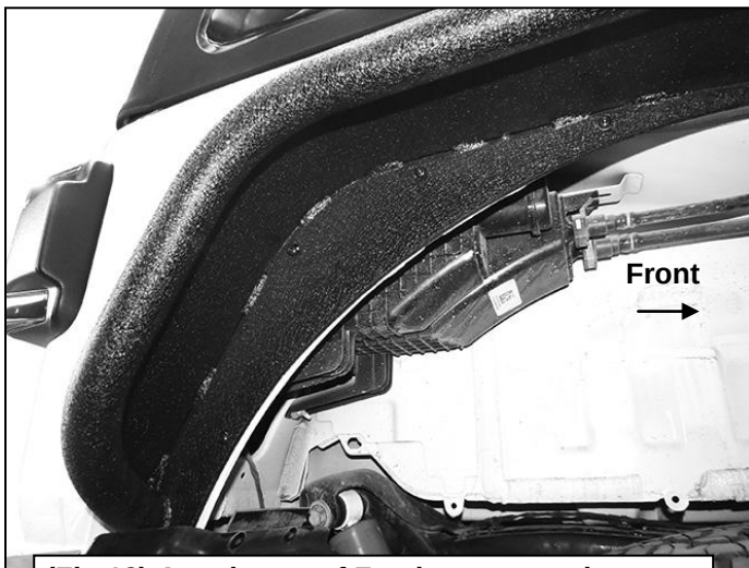
(Fig 13) Attach rear of Fender to mounting locations on body, (driver/left Fender pictured)
