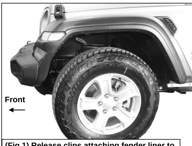
(Fig 1) Release clips attaching fender liner to outer fender
