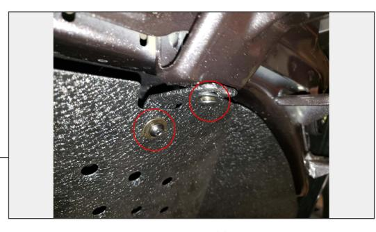
Attach the upper fender bracket to the fender mount using the (1) M10x1.50x25mm Allen bolt, lock washer, flat washers, and nuts. Then attach the upper portion of the fender liner to the upper fender bracket using (1) M10x1.50x25mm Allen bolt, lock washer, and flat washer.
