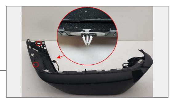
Remove the (2) plastic push clips shown in the picture above using a flat head screw driver.
