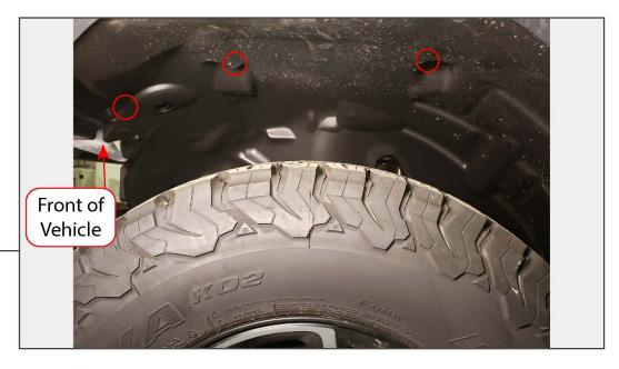
Located and remove the (3) 10mm screws securing the front portion of the front fender liner in place. Then, fully remove the fender liner from the vehicle.
