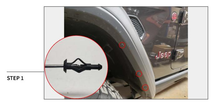
Begin by removing the factory fender liners by removing the (3) plastic pop rivets located above by using a small Phillips head screw driver and pushing the center of the rivet through.
