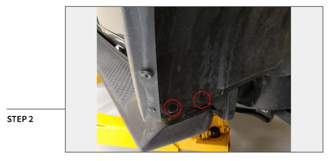
Using a trim panel removal tool, locate and remove the (2) lower push clips securing the back portion of the front fender liner in place.
