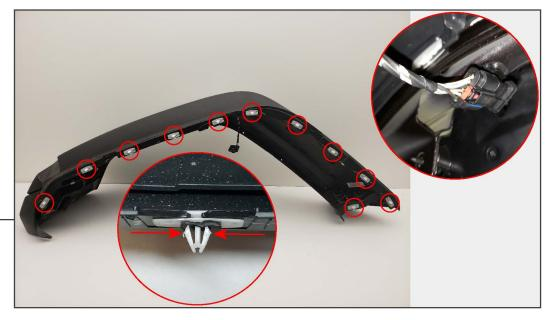
Locate, and unplug the fender wiring plug connector. Then locate and carefully depress the (11) plastic push clips using a trim panel removal tool, and remove the fender from the vehicle.
