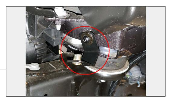
Attach the lower body bracket to the speed clip that was installed in the last step using (1) M10x1.50x25mm Allen bolt, lock washer, and flat washer.
