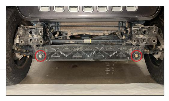
Remove (2) 16mm bolts from the lower metal shield, then lift upwards to unhook the shield from the vehicle.
