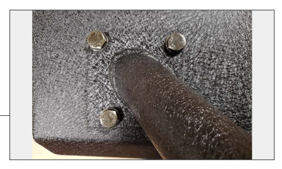
Install the optional over-rider light bar mount or the (2) block off plates to the bumper by using the (6) M10 x 1.50 x 25mm bolts, (12) M10 flat washers, (6) M10 lock washers, and (6) M10 nuts.
