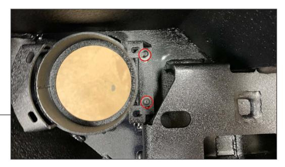
Using (2) M4 bolts, (2) M4 lock washers, and (2) M4 flat washers, attach the fog light bracket to the bumper. Repeat on both sides of the bumper.
