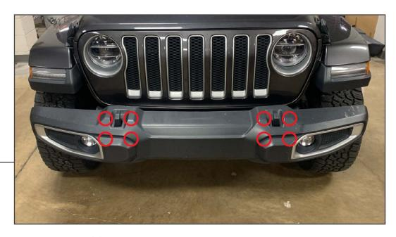
From behind the bumper, remove (8) 18mm nuts to release the bumper from the vehicle frame. Once all hardware is removed, pull the bumper away from the vehicle and place on a workable surface.
