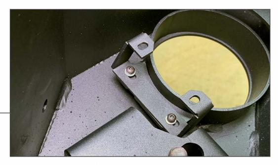
Using (2) M4 bolts, (2) M4 lock washers, and (2) M4 flat washers, attach the fog light bracket to the bumper. Repeat on both sides of the bumper.
