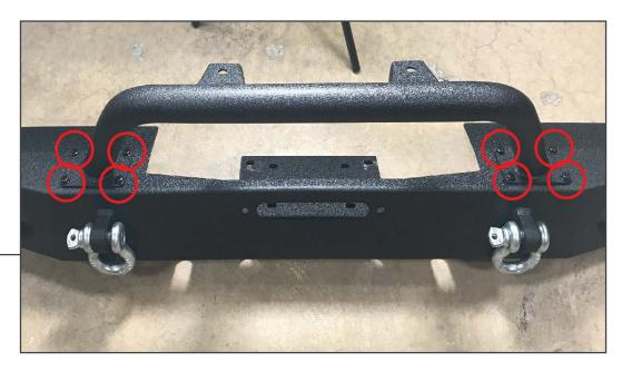
Install the over-rider bar onto the bumper using (8) M8x1.25x25mm bolts, (16) M8 flat washers, and (8) M8 nuts. Tighten the mounting hardware evenly until the over-rider is secure.
