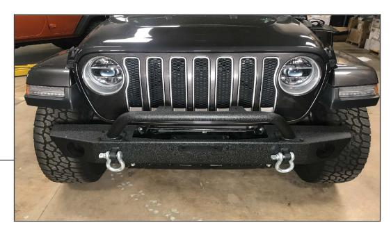
With help, carefully install the bumper to the vehicle. Secure the bumper to the vehicle using the provided M12 hardware. Re-connect the fog lights using the original bumper harness (extending the harness may be necessary).
