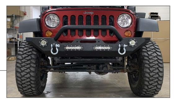
Neatly route the wiring harnesses away from any hot/moving components using cable ties. Install the (2) 3/4" D-Rings into the bumper mounting points, if desired.
