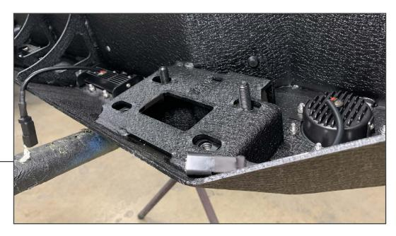
Fit (2) M12 stud plates behind the bumper mounting pad on each side of the bumper. The studs will fit through the vehicle frame rails.
