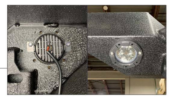
Fit each LED light into the bumper assembly. While holding the front trim panel in line with the bolt holes, fit (2) M6 Allen bolts through the trim panel, bumper, and LED light brackets. Loosely secure using (2) M6 lock nuts.
