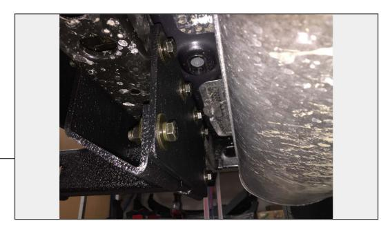
Install the hitch assembly and hitch plate using the (4) M12  $\times$  120mm bolts, and (2) M12  $\times$  40mm bolts, flat washers, and lock washers. Torque to 40 ft-lbs.
