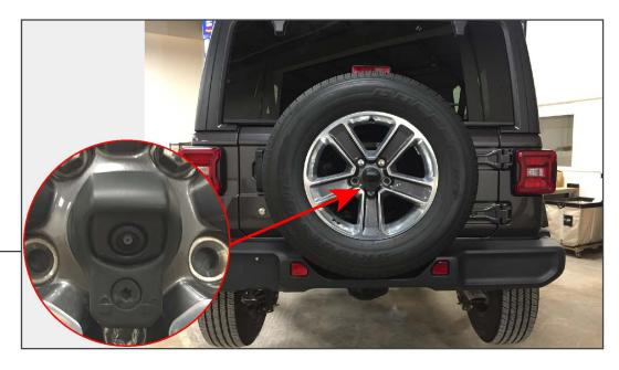
Locate the T-40 Torx lock screw on the camera cover, and turn it counter-clockwise to unlock. Remove the camera cover by pulling away from the vehicle. Then, remove the (3) lug nuts to remove the spare tire.
