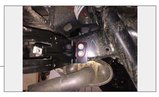
Once the splash shields are removed, locate and remove the (2) 16mm bolts securing the splash shield brackets to the bumper. Bumper will now be loose.
