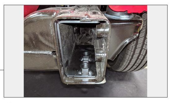
Insert the supplied (1) dual nut plate into the passenger side frame rail over the lower frame holes.
