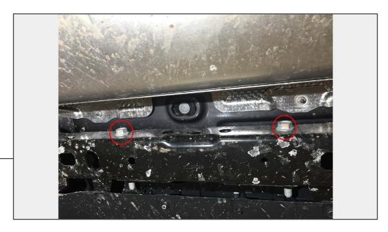
From directly under the center of the vehicle, locate and remove the (2) 16mm bolts supporting the center of the bumper to the vehicle frame.
