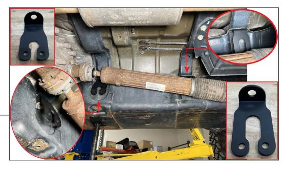
Locate and remove (2) 18mm bolts along the side mounts of the fuel tank. With the bolts removed, fit the appropriate included mounting brackets and loosely secure using the original (1) 18mm bolt per bracket.
