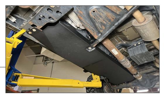
Ensure all fuel tank and skid plate hardware is fully tightened.
