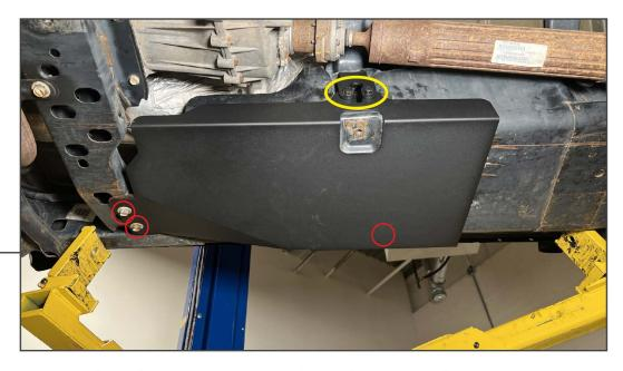
With a floor jack or helper, lift the front skid plate to the front of the vehicle fuel tank. Loosely secure the skid plate to the fuel tank using the original (3) 18mm bolts.
