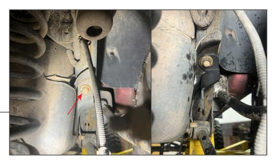
Locate and remove (1) 18mm bolt at the rear mounting point of the fuel tank. With the bolt removed, fit the appropriate included mounting bracket and loosely secure using the original (1) 18mm bolt.
