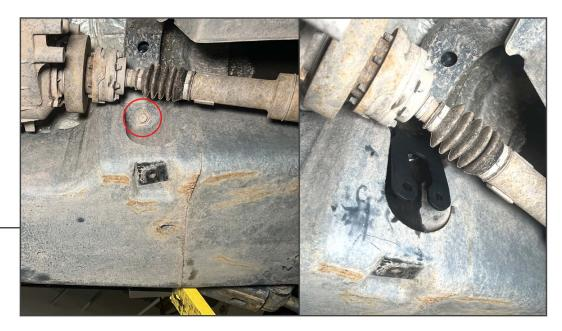
Locate and remove (1) 18mm bolt at the front-most side mounting point of the fuel tank. With the bolt removed, fit the appropriate included mounting bracket and loosely secure using the original (1) 18mm bolt.
