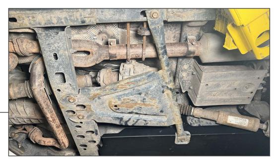
Tighten all fuel tank mounting bolts to the vehicle, then tighten the skid plate M12 bolts into the mounting brackets.
