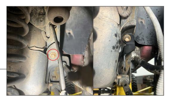
Locate and remove (1) 18mm bolt at the rear mounting point of the fuel tank. With the bolt removed, fit the appropriate included mounting bracket and loosely secure using the original (1) 18mm bolt.
