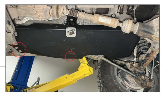
With a floor jack or helper, lift the skid plate to the vehicle fuel tank. Loosely secure the skid plate to the fuel tank using the original (3) 18mm bolts.
