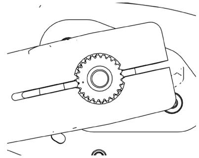
Make sure the gap in the arm aligns with the dot on the bar.
