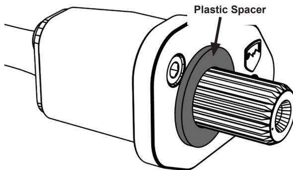
Spacers can be configured to set the arm closer to the frame or the tire depending on your needs. Put the arm away from the tire (closer to the frame) unless it will rub on an aftermarket inner fender liner.
