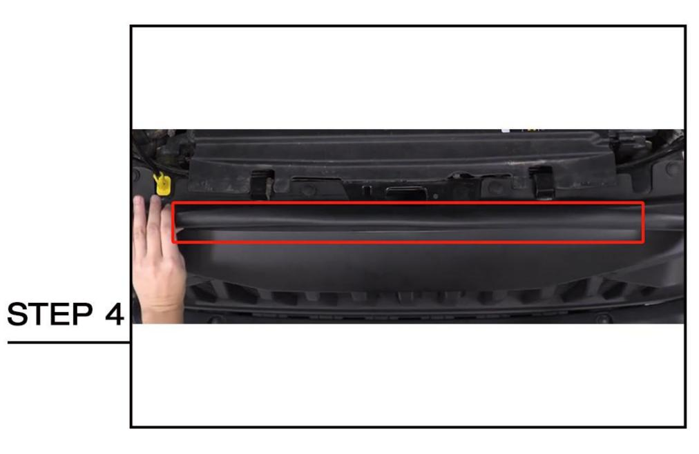
Align the grille to the car and get the retainer clips in the right position. Apply the supplied weather stripping accross the black wire to the negative terminal. the top of the grille.
