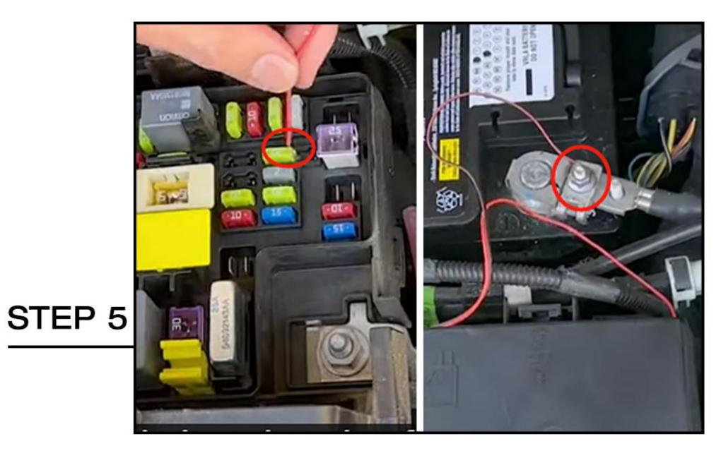
Open the fuse box, connect the red wire to the ACC,
