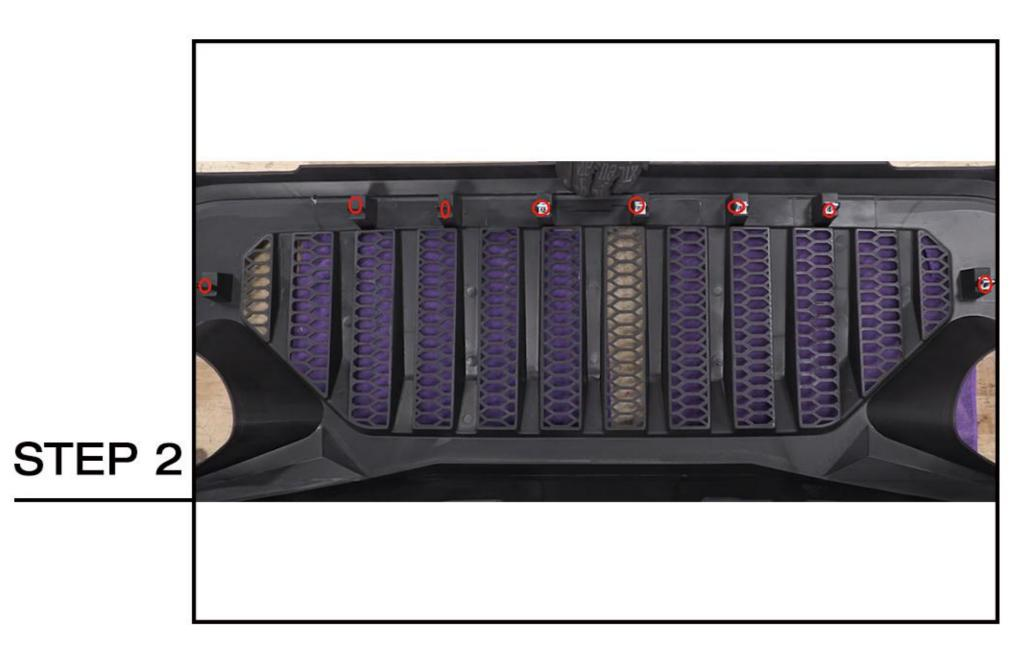
Install 8 retaining clips in the appropriate position on the back of the grille.
