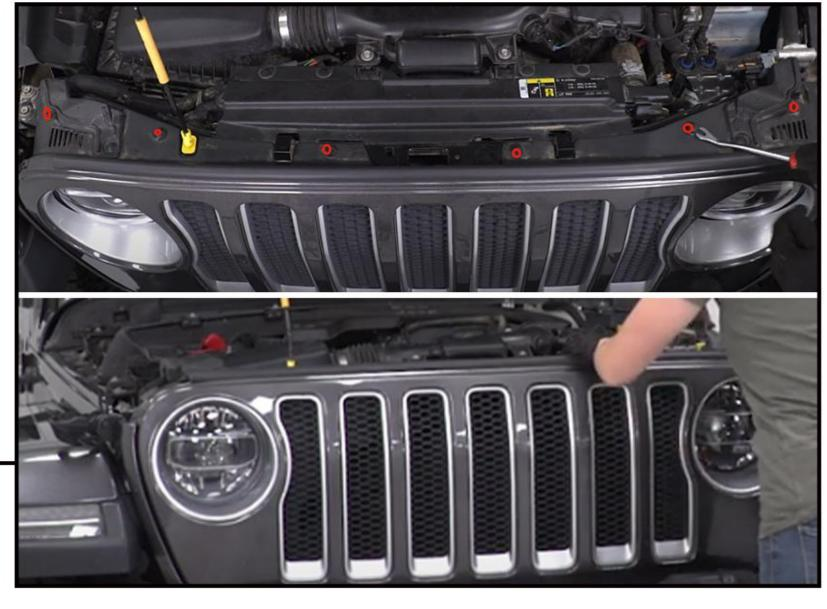
Open the hood, remove 6 push clips at the top of the grille, then pull the two lower corners to release clips and remove the grille.
