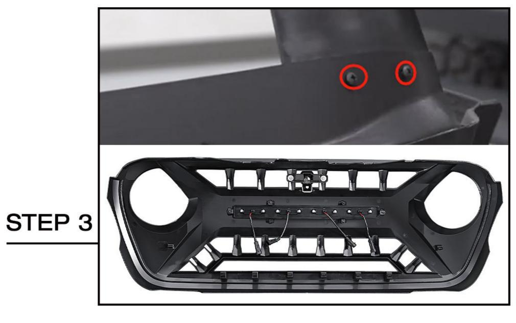
Fixed the bracket with the screws on both sides. If your car is equipped with a camera, please remove the cover plate on the new grille and install the camera bracket. (There is a camera bracket included in the accessories)
