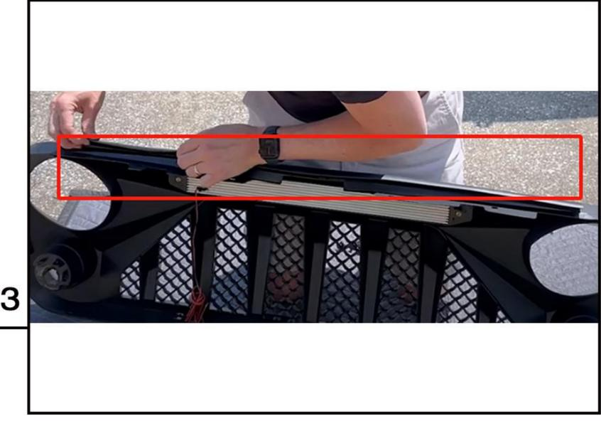
Pop the hood, remove the 6 push clips with a panel removal tool; Unplug the turn signals and pull the grille out of the car.
