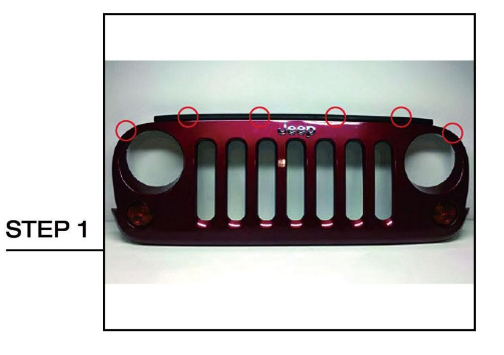
Using a panel removal tool, remove the (6) push
