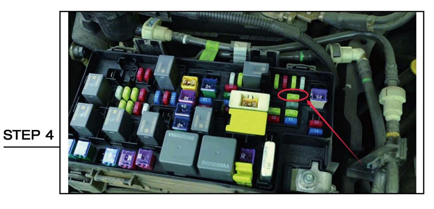
Connect the red and black wire of the light bar to ACC and negative of battery.
