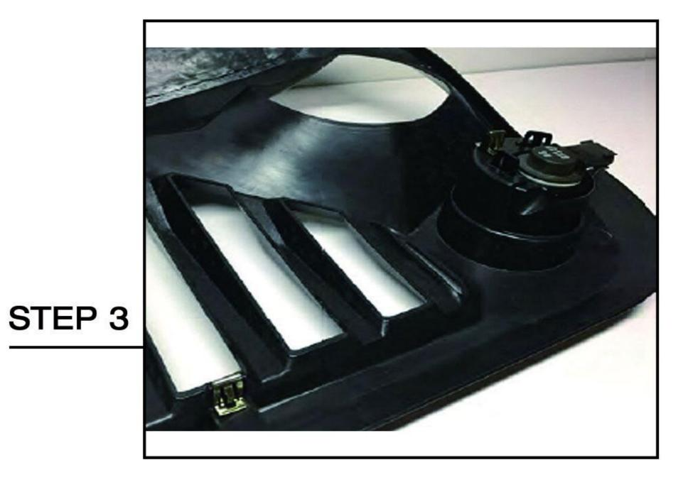
Press on the (6) supplied retaining clips. Using the factory grilleas a reference, apply the supplied weather stripping acrossthe top of the grille.
