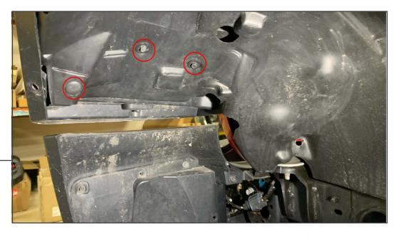
Fold back the fender liner to access the fender marker light wiring. Remove the (2) 8mm screws and (1) push clip.
