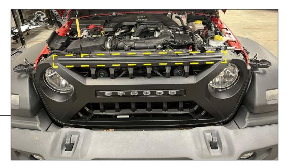
Clean the top edge of the grille using isopropyl alcohol and a microfiber cloth. Close the hood to visualize the weatherstripping mounting location. Once familiar, peel the red tape backing from the weatherstripping and adhere the weatherstripping to the grille. Firmly press into place until secure.
