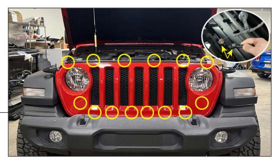
Using a soft pry tool, remove the (6) plastic push pins across the top of the factory grille. Then, firmly pull the grille away from the vehicle to dislodge the (8) retaining clips along the bottom of the grille.
