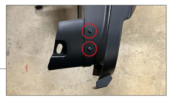
Secure each grille upper mounting bracket to the backside of the grille using (2) Phillips screws [Black].
