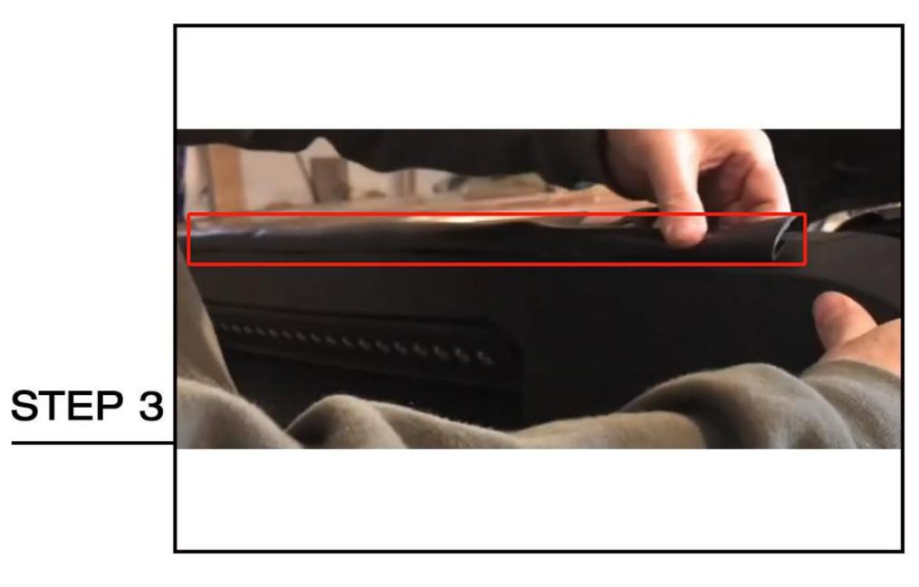
Apply the supplied weather stripping accross the top of the grille. Put all the clips on the grille and reinsert the turn signal cups.
