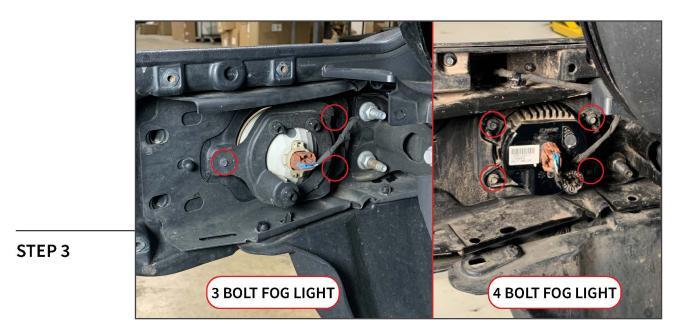
Depending on vehicle trim level, remove the (3) OR (4) 7mm fog light retaining bolts and remove the fog light from the vehicle. Install the new LED fog light with the appropriate mounting adapter to the vehicle bumper reusing the original hardware, and plug in the vehicle wiring harness.
