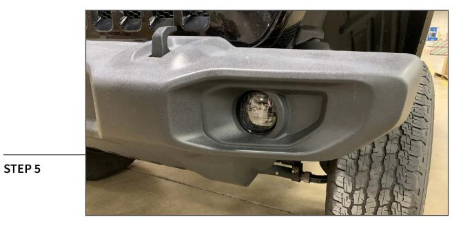
Adjust the fog lights using the attached Allen bolt.
