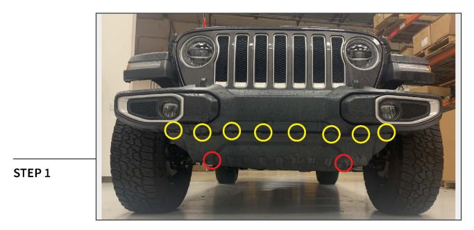
Remove (2) 8mm bolts from the plastic lower shield, then remove (8) plastic push clips. Remove the plastic lower shield from the vehicle.
