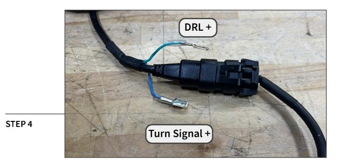
Plug the (2) wire leads into each fog light spade connector. Then, route the wire leads towards the vehicle fender flare turn signal/parking lamp. Using the (2) scotchlok connectors, splice the wire leads into the vehicle wiring harness. Use a test light/multimeter to verify connections before splicing.
