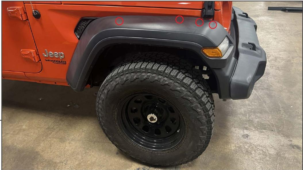
Remove (4) 10mm bolts from the inside of the fender flare.
