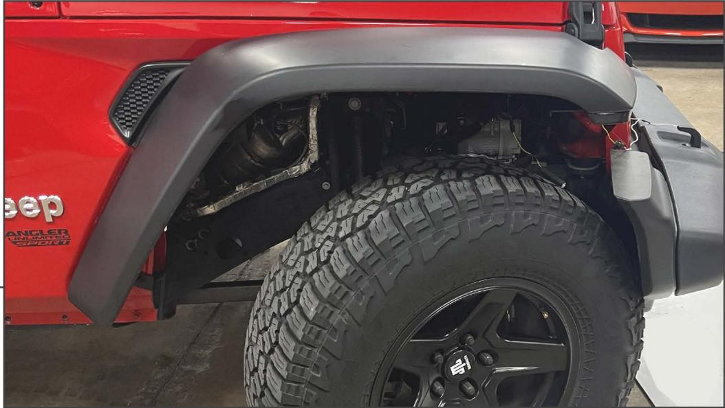
Repeat steps 1-6 for the remaining front fender flare. Route the DRL harness across the front of the vehicle, and plug the DRL harness into the flares. Route the fuse lead towards the vehicle fuse box. Splice the fuse tap into a ignition (key on) power circuit in the fuse box.
