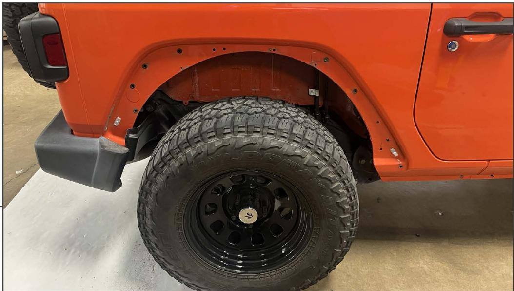
Remove (5) plastic push clips from the vehicle fender flare/liner. Then, firmly pull the flare from the vehicle.
