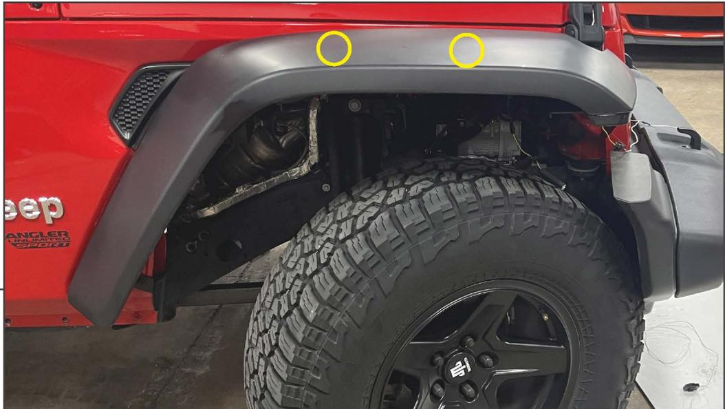
Secure the center of the fender flare to the fender using (2) M8 x 25mm flange bolts and (2) M8 flat washers.
