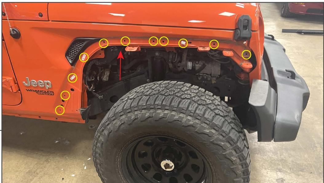
Firmly pull the fender flare away from the vehicle to disengage the plastic retaining clips along the edge of the flare. Once pulled away slightly, unplug the vehicle flare electrical connector.
