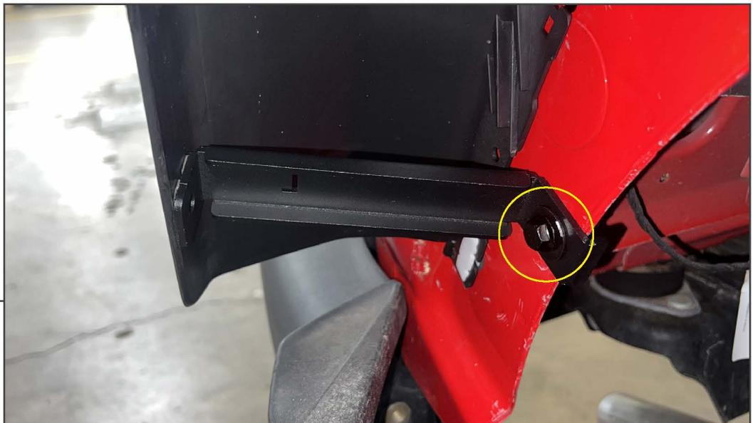
Fit (1) M6 threaded insert into the vehicle body. Then, secure the rear bracket to the vehicle body using (1) M6 x 25mm bolt. Then, remove the double sided tape backing from the bracket and adhere the bracket to the fender flare.
