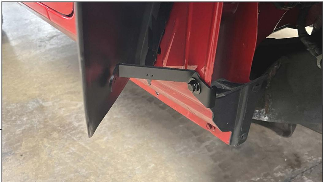
Using the rear bracket, secure the bracket to the vehicle fender using (1) M8 x 25mm bolt, (1) M8 flat washer, and (1) M8 flange nut. Then, remove the double sided tape backing from the bracket and adhere the bracket to the fender flare.
