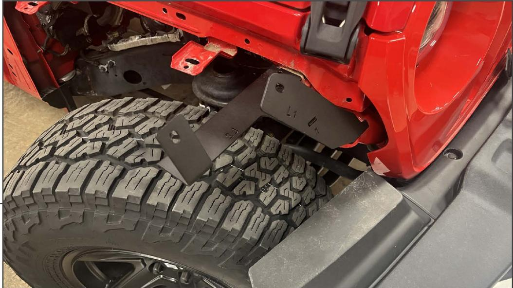
Fit the front mounting bracket to the fender mounting points, and secure using (2) M8 flange bolts, (2) M8 flat washers, and (2) M8 flange nuts. Do not fully tighten at this time to allow for later adjustments.
