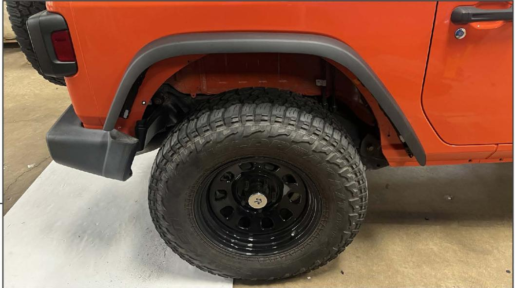
Install the included (12) plastic retaining clips to the edge of the new fender flare. Then, fit the fender flare to the vehicle by manipulating the flare to align all the plastic clips to the vehicle holes.
