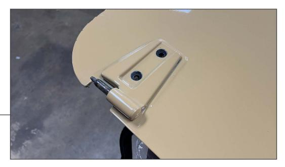
Remove (2) T-50 Torx bolts from each door hinge. Lift and remove the hinge from the vehicle.
