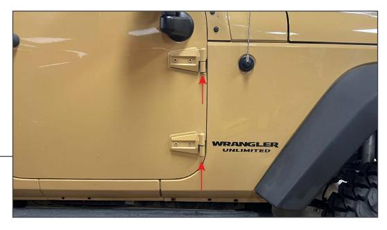
\*\*Removing and installing door hinges to the vehicle will effect the door alignment to the vehicle. Aligning the door properly can be difficult, and this can lead to vehicle damage if done incorrectly. Professional installation is recommended by a qualified auto body shop.
