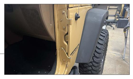
Remove (3) 13mm bolts from the upper inner door hinge. Lift and remove the hinge from the vehicle.
