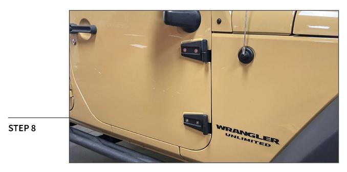
Repeat steps 1-7 for all remaining door hinges. Install the OEM T-50 nuts onto the bottom of the new hinges to lock the door pins.
