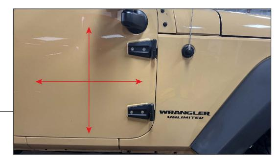
Lift the door to the vehicle and carefully place the door onto the new hinges. Verify clearances between the hinges and the door to prevent door damage. Slowly close the vehicle door, checking clearances and body gaps around the door, while ensuring door striker alignment.
