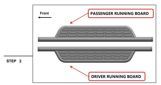
Identify each running board by identifier on the front. Notice: "D" for Driver/Left Side; "P" for Passenger/Right Side.
