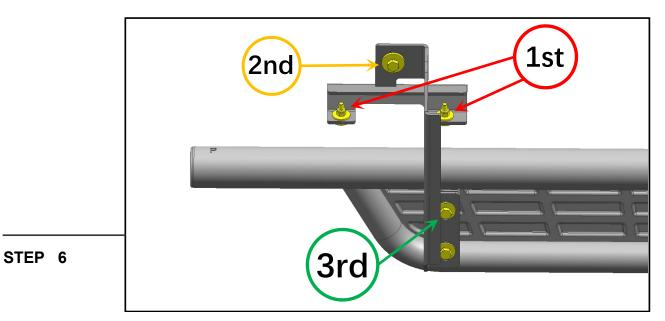
Tighten the mounting brackets to the vehicle (M6 first, then M8). Adjust the running board to the desired angle, and tighten the M8 combo bolts to secure the step into place. See photo for tightening order visual.
