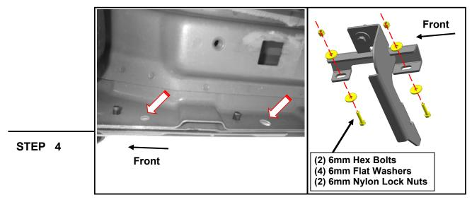
Loosely fit the Passenger Front bracket to the vehicle pinch weld using (2) M6 x 25mm hex bolts, (4) M6 flat washers, and (2) M6 nylon lock nuts. Do not fully tighten to allow for later adjustments. Repeat this step for all step brackets.
