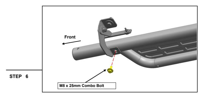
With all brackets loosely mounted to the vehicle, fit the running board onto the brackets, and loosely secure into place using (3) M8 x 25mm combo bolts.
