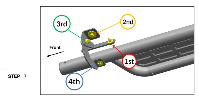
Tighten the mounting brackets to the vehicle (M6 first, then M8 / M10). Tighten the M10 bolt joining the brackets together. Adjust the side step to the desired angle, and tighten the M8 combo bolts to secure the step into place. See photo for tightening order visual.
