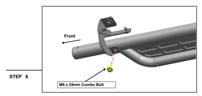
With all brackets loosely mounted to the vehicle, fit the running board onto the brackets, and loosely secure into place using (5) M8 x 25mm combo bolts.
