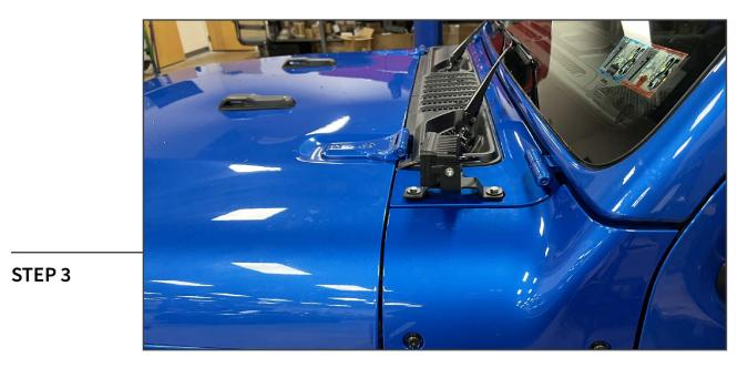
With the spacers in place, align the LED light & bracket assembly to the cowl. Secure the lighting into place using the included (2) M6 x 50mm Allen bolts, (2) M6 lock washers, and (2) M6 flat washers. Tighten the hardware evenly until secure. Route the LED light connector into the engine bay away from any moving components.
