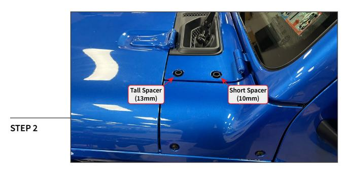
Identify the included spacers. The taller (13mm) spacer fits into the front cowl bolt hole. The shorter (10mm) spacer fits into the rear bolt hole.
