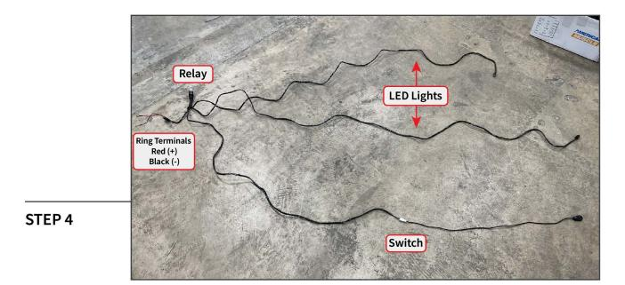
Lay out and identify the components of the included wiring harness.
