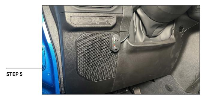
Test fit the switch to a desireable location on the dashboard. Clean the area using isopropyl alcohol and a microfiber cloth, and allow to fully dry. Once dry, remove the tape backing and firmly press the switch into place to encourage adhesion.
