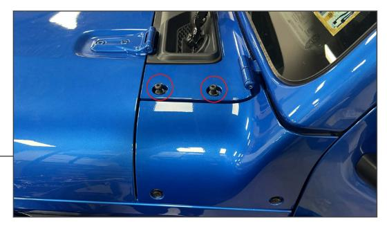
In between the vehicle hood and windshield, locate the (2) T-40 Torx bolts securing the cowl to the vehicle. Remove the (2) T-40 Torx bolts.
