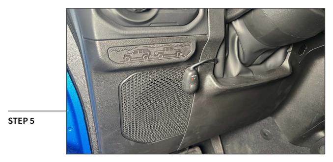
Test fit the switch to a desireable location on the dashboard. Clean the area using isopropyl alcohol and a microfiber cloth, and allow to fully dry. Once dry, remove the tape backing and firmly press the switch into place to encourage adhesion.
