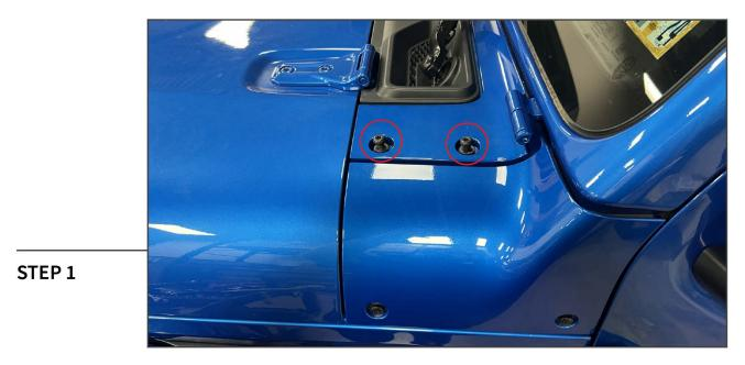
In between the vehicle hood and windshield, locate the (2) T-40 Torx bolts securing the cowl to the vehicle. Remove the (2) T-40 Torx bolts.
