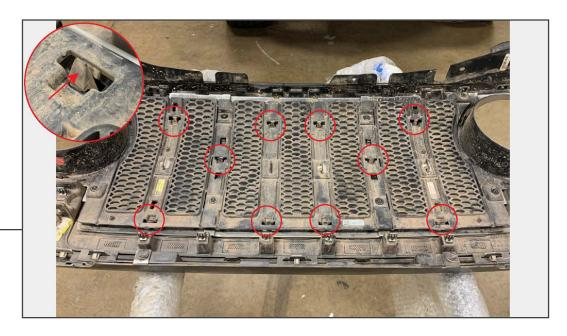
Gently pry back on the grille insert retaining tabs to release the inserts from the grille assembly.
