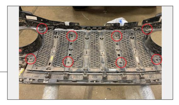
Remove the (8) T-20 Torx bolts from the back of the grille.
