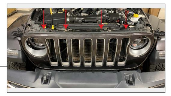
Loosely fit the grille to the vehicle. Place the grille insert in between the vehicle and the grille through the top.
