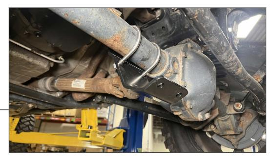
Loosely install the (1) axle mounting bracket to the axle tube using (2) large U-Bolts and (4) 3/8-16 flange nuts.
