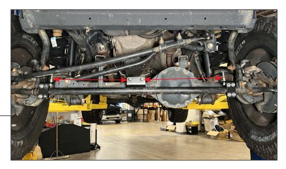
Fit (2) 1/2-13 bolts and (2) 1/2-13 flat washers into the axle mounting bracket. With the wheels straight, measure the distance from the axle mounting bracket bolts to the tie rod mounting bracket studs. Each side will measure approximately 16".
