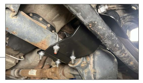
Begin tightening the stabilizer assembly by lifting the bracket adequately clearance the tie rod. Tighten the (4) 3/8-16 flange nuts evenly until the bracket is secure.
