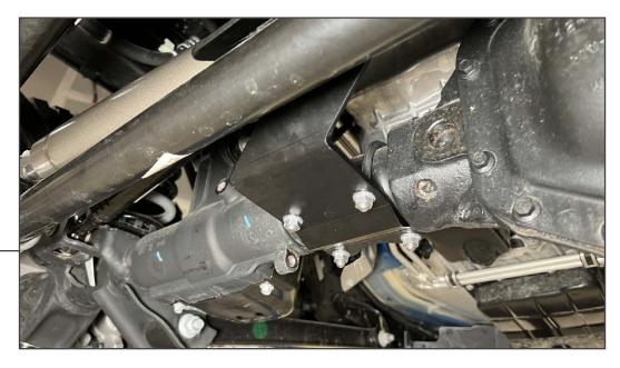
Begin tightening the stabilizer assembly by lifting the bracket adequately clearance the tie rod. Tighten the (4) 3/8-16 flange nuts evenly until the bracket is secure.
