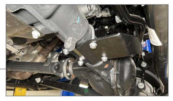
Loosely install the (1) axle mounting bracket to the axle tube using (2) large U-Bolts and (4) 3/8-16 flange nuts.
