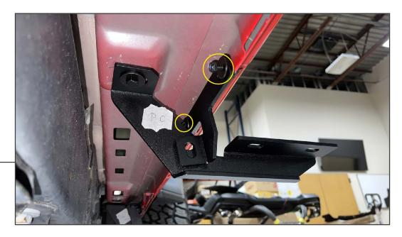
Loosely secure each appropriate rocker panel mounting bracket to the vehicle using (2) M6 x 25mm bolts, (4) M6 flat washers, and (2) M6 lock nuts through the vehicle pinch weld.
