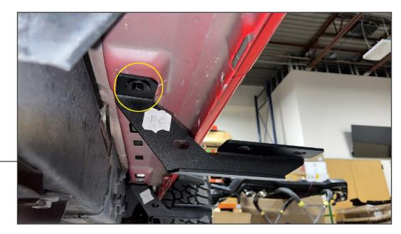
Loosely secure each appropriate step mounting bracket to the vehicle using (1) M8 x 35mm bolt, (1) M8 lock washer, and (1) M8 flat washer into the vehicle threaded insert.
