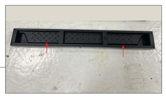
Fit (2) stud plates onto the inside of the side step. Then, fit the side step to the brackets, ensuring the studs align within each mounting bracket.
