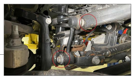
Safely lift and support the front of the vehicle off the ground using a floor jack and jack stands. With access under the vehicle, remove the (2) 18mm nuts/bolts from each of the original sway bar links.
