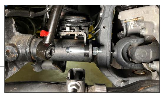
Secure the (1) lower sway bar link mount to the vehicle axle using the included lock nut. Fit a small hand tool through the hole in the mount to hold the mount while tightening the lock nut.
