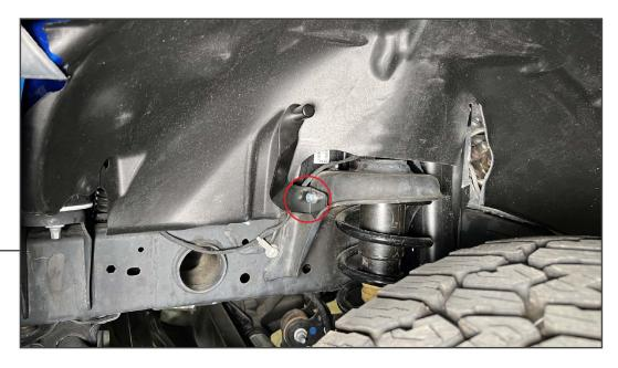
Using the included M8 hardware, secure the sway bar link retaining brackets to the vehicle coil spring mount. This bracket will retain the sway bar links when the sway bar links are disconnected. Secure the sway bar links to the bracket using the lower mount click pins.
