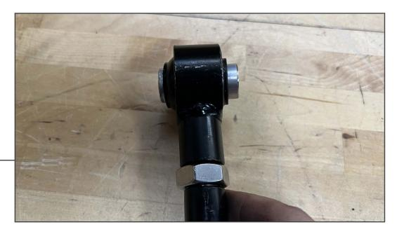
Using a hammer, fit the M12 sleeve into the top of the sway bar link.
