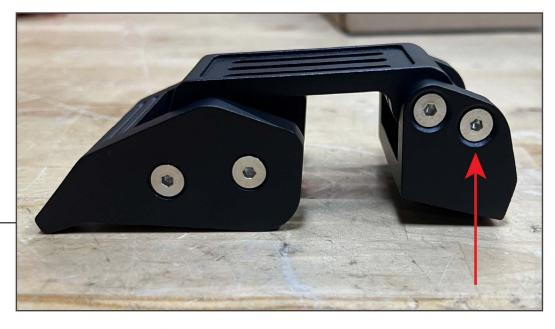
Place the hood catch on a workable surface. Using a 3mm Allen key, remove the hood catch limiting bar temporarily.
