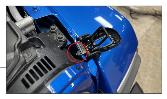
Open the vehicle hood, and locate the hood catch stud. Remove (1) 13mm nut from the hood catch, then remove the hood catch.
