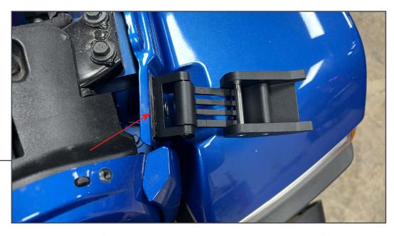
Mount the fender mounted portion of the hood catch and appropriate spacer using (1) M8 Allen bolt, (1) M8 flat washer, and (1) M8 lock nut. Ensure the spacer is fully seated into the fender holes and the hood catch is pointing upwards while tightening.
