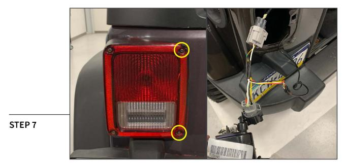
Remove (2) Phillips head screws to remove the vehicle tail light assembly from the vehicle. Once removed, unplug the tail light assembly. Install the included in-line adapter harness to the vehicle wiring harness and the tail light assembly. Plug in the roof mounted tail light.
