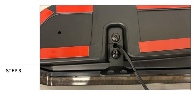
Install the tail light bracket to the light housing using (2) M6 x 12mm Phillips bolts, (2) M6 lock washers, and (2) M6 flat washers. Tighten until secure.
