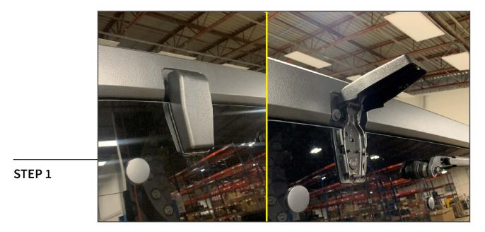
Using a plastic pry tool, gently pry the hinge covers from the rear glass hinges, starting from the bottom. The cover will hinge upward once dislodged. Remove the hinge cover from the vehicle.
