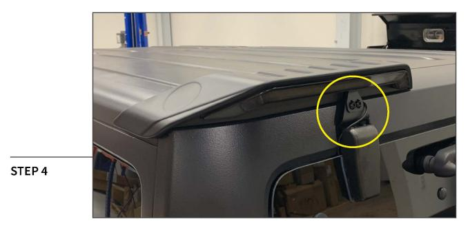
Clean the roof of the vehicle using the included adhesion promoter pads. Once clean and dry, remove the double sided tape backing from the light and adhere the light to the vehicle. Secure the light assembly to the vehicle hardtop using the original (2) 10mm bolts.
