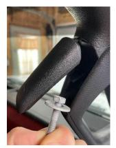
Using a 10mm socket and extension, loosen up the top bolt and remove the bottom bolt. Save the bottom bolt with the bottom cover. The mirror mounts come with longer bolts to be used in the bottom hole.
