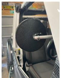
Once you have the mount secure to the Jeep you may slide the mirror into the mount and tighten the thumb screw at the desired spot. The mirrors will not stick out far past the windshield frame. The convex shape of the mirror helps you see what you are beside without sticking way out like a traditional mirror would be. Make sure you rotate the mirror 180 degrees from the way they are packaged. (See bottom photo on left) Note: The mirrors are the same, the mounts are different.
