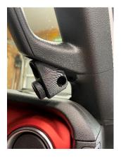
Take passenger side mount and push it into the hole as shown in the picture. (it will be a snug fit, designed like this on purpose to keep any vibration down) Take new supplied bolt and thread the bolt into the mount. Once you have the bolt into the threads on the jeep tighten up the top and the bottom bolts and pop top cover back into place. (If you have trouble getting the bottom bolt started, take the top bolt completely out so the handle can move around a bit more.)
