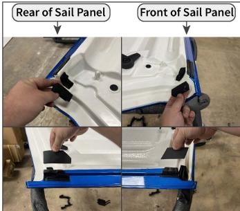
Identify the mounting location for each of the provided hardtop/sail panel seals using the diagrams above. Once familiar with location, remove the original seal and clean the area using isopropyl alcohol to remove all of the original adhesive.
