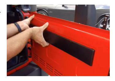
**Step 5:** Route the harness's black barrel connector into the hold behind the trim panel from the swing gate.
