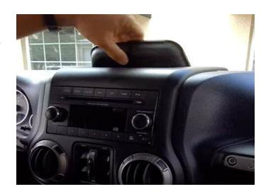
**Step 18:** Remove the one 7mm screw from under the rubber mat.
