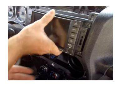
**Step 33:** Secure the radio in place with the four screws.
