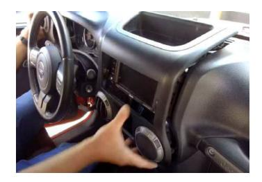
**Step 35:** Install the four 7mm screws back into place to hold the bezel securely.
