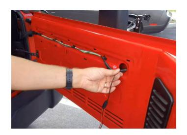
**Step 6:** Connect the barrel connector to the other end of the barrel connector from the camera side.
