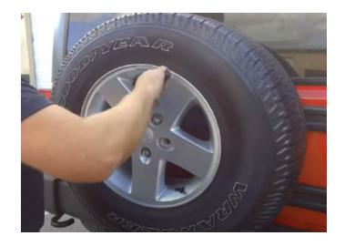
**Step 2:** Slide on the camera bracket. Secure with lug nuts for now.
