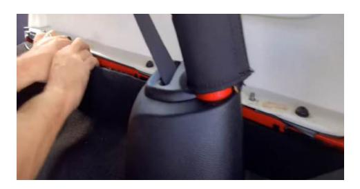
**Step 15:** Continue to route the harness down and along the trim panels going toward the front of the vehicle.
