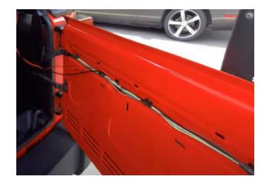
**Step 8:** Wrap the harness to the factory wiring going into the vehicle.
