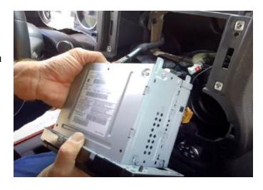
**Step 32:** Push the radio back into place. Make sure not to pinch or break any of the connections. Don't force the radio in.
