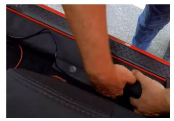
**Step 17:** Now we need to get to the rear of the radio to install the interface harness. This will allow us a RCA connection to the OEM radio for the video signal input from the backup camera. Remove the rubber mat from above the radio.
