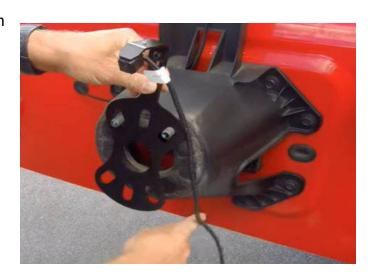
**Step 3:** Put your lug nuts on to hold bracket from falling off. Route the cable through to hold circled in yellow.
