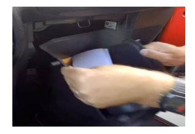
**Step 26:** Route the harness behind the glove box and into the cavity behind the radio. Zip tie any of the harness out of the way that is left so it doesn't interfere with the glove box operation.
