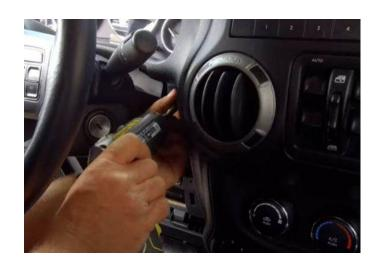
**Step 21:** Next remove with pry tool the window controls. There is a small red tab that needs to be pushed up then depress the button to release the window controls. Remove the one 7mm screw behind the window controls.
