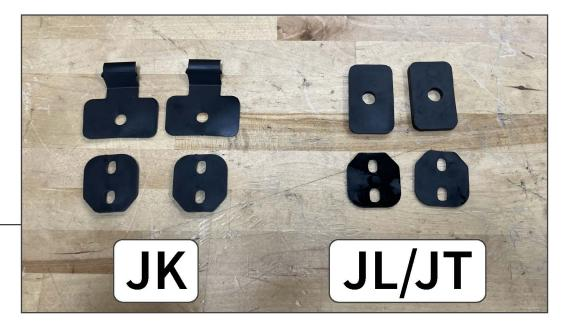
Lay out and identify the included rubber gaskets. Depending on the vehicle, the appropriate gaskets will be used.
