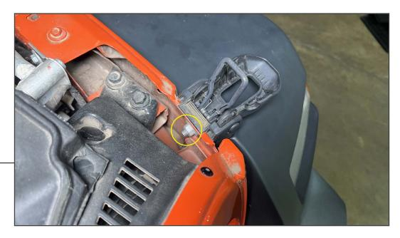
Open the vehicle hood. Remove (1) 13mm nut from the hood latch base. Remove the hood latch base from the vehicle.
