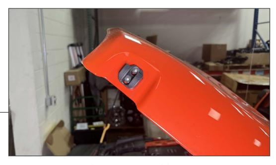
Using (2) M6 x 20mm tapered Allen bolts, (2) M6 flat washer, and (2) M6 lock nuts, secure the hood catch to the vehicle hood. Ensure the included appropriate gasket is between the hood and the catch.
