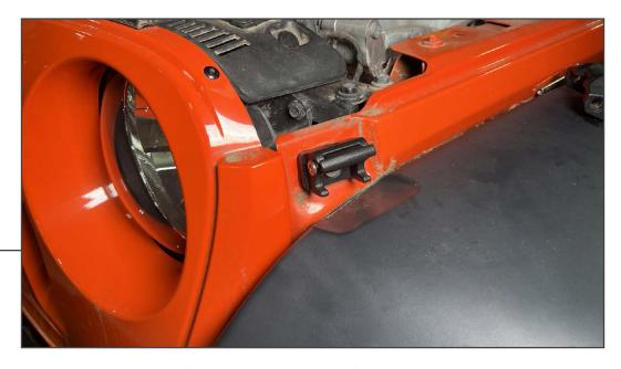
Using (1) M8 x 20mm tapered Allen bolt, (1) M8 flat washer, and (1) M8 lock nut, secure the hood latch base to the vehicle fender. Ensure the included appropriate gasket is between the fender and the hood latch base.
