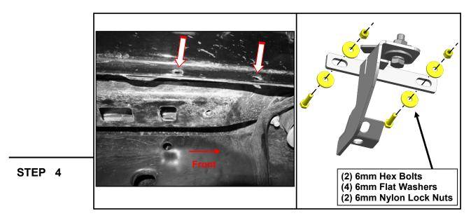
Loosely fit the Passenger Front bracket to the vehicle pinch weld using (2) M6 x 25mm hex bolts, (4) M6 flat washers, and (2) M6 lock nuts. Do not fully tighten to allow for later adjustments. Repeat this step for all step brackets.
