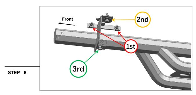
Tighten the mounting brackets to the vehicle (M6 first, then M8 / M10). Adjust the running board to the desired angle, and tighten the M8 combo bolts to secure the step into place. See photo for tightening order visual.
