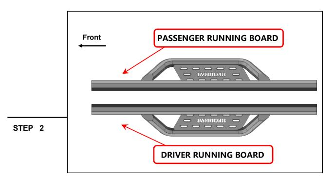
Identify each running board by identifier on the front. Notice: "D" for Driver/Left Side; "P" for Passenger/Right Side.
