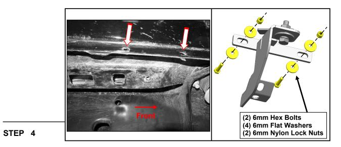
Loosely fit the Passenger Front bracket to the vehicle pinch weld using (2) M6 x 25mm hex bolts, (4) M6 flat washers, and (2) M6 lock nuts. Do not fully tighten to allow for later adjustments. Repeat this step for all step brackets.
