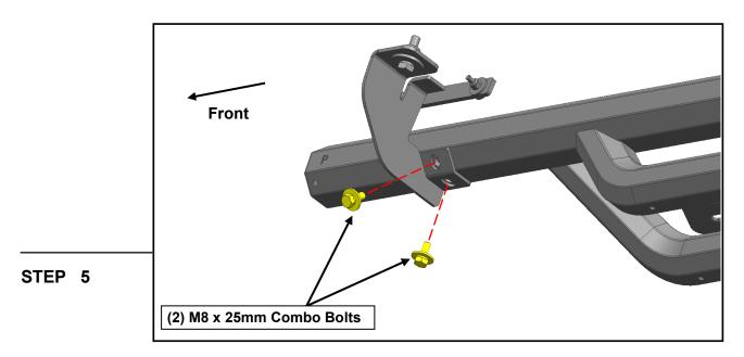
With all brackets loosely mounted to the vehicle, fit the running board onto the brackets, and loosely secure into place using (4) M8 x 25mm combo bolts.
