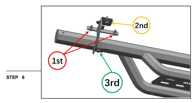
Tighten the mounting brackets to the vehicle (M6 first, then M8 / M10). Adjust the running board to the desired angle, and tighten the M8 combo bolts to secure the step into place. See photo for tightening order visual.
