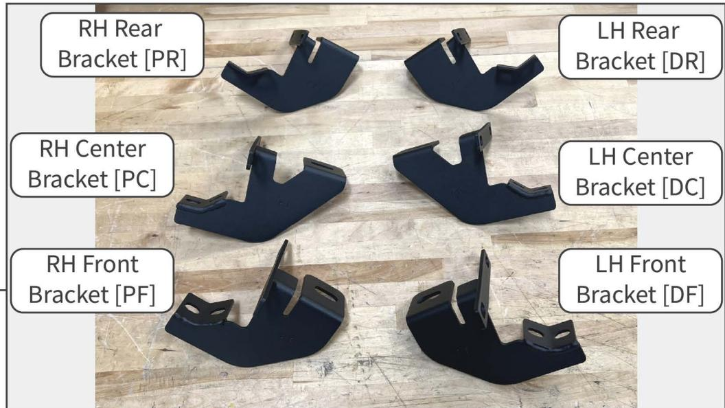
Locate the identification label on each mounting bracket.
