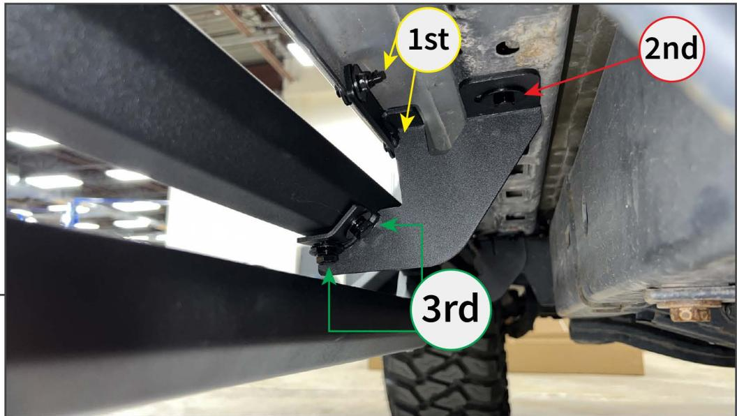
Adjust the drop step and bracket for the desired fit to the vehicle. Tighten all hardware following the diagram above.
