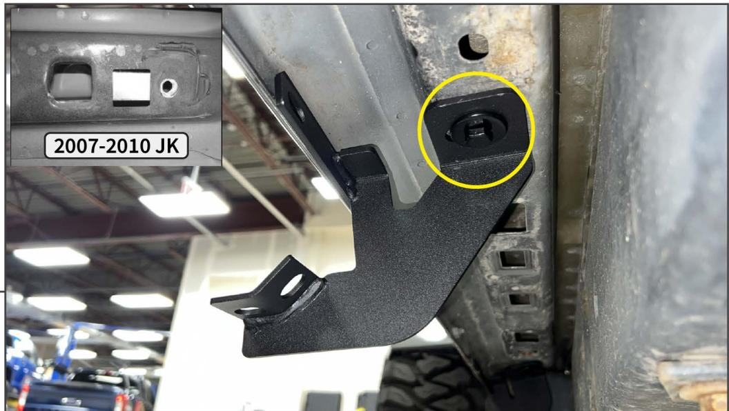
Align each appropriate mounting bracket to the vehicle body, and loosely secure the rear of each mounting bracket using (1) M8 x 35mm bolt, (1) M8 lock washer, and (1) M8 flat washer.
