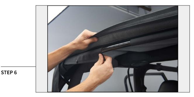
Raise the top toward the windshield and lock it into place. Then, snap the fabric onto the rear bow.
