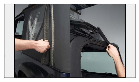
Remove factory quarter and rear windows, uninstall the tailgate bar attached to the bottom of the rear window from the plastic clamps. Next, unlatch the plastic tabs holding the top to the door channels by pulling down and away from your Jeep and unhook the windshield latches, freeing the top from the windshield.
