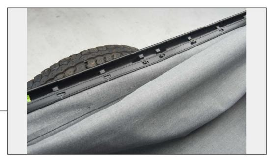
With both the center and rear bows laying down on the rear of the vehicle, lay the fabric over the top with the backing side up. Line the plastic strip up with the edge of the header and using the center hole, screw the fabric down. After the center is secure, you can then proceed to secure the rest of the plastic strip.
