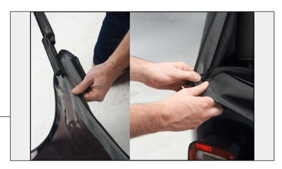
Install the tailgate bar onto the rear window and insert the assembly into the mounts with the vinyl side out. Zip up the window and cover the zipper ends with the overlapping fabric from the rear corners attached in Step 8.
