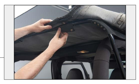
Unhook the factory top from the rear bow by unsnapping it. Next, unhook the center bow flap to completely separate the top from the frame.
