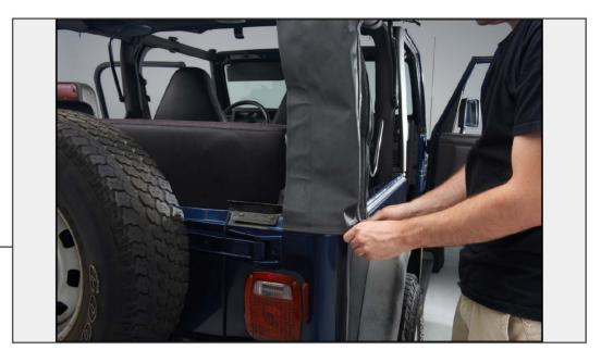
Pull down the rear corners of the top, and secure the corners to the vehicle, then close the header latches. \*Depending on how tight your top is, it may help to release the windshield latches, and or let the top sit outside in the sun.
