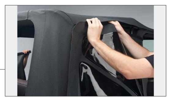
Install the quarter windows by zipping them into place. Then secure the plastic strips into the channels on the body and door surround.
