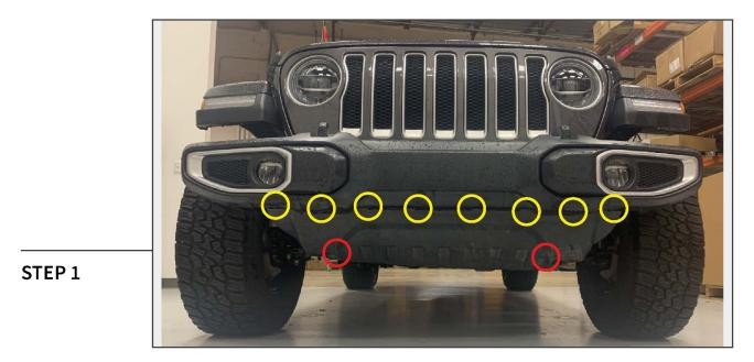
Remove (2) 8mm bolts from the plastic lower shield, then remove (8) plastic push clips. Remove the plastic lower shield from the vehicle.
