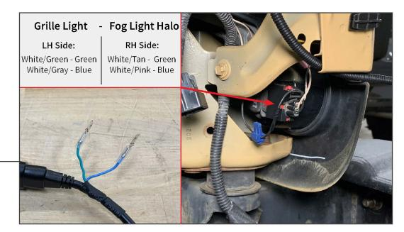
Plug the fog light into the vehicle fog light wiring harness. Test Halo functionality, and splice the additional wire leads into the grille mounted parking/turn signal lamp following the diagram above using the included (2) scotchlok connectors.
