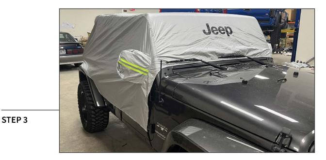
Using the (8) attached elastic hooks, attach the cover to a suitable location under the vehicle, and tighten to secure.
