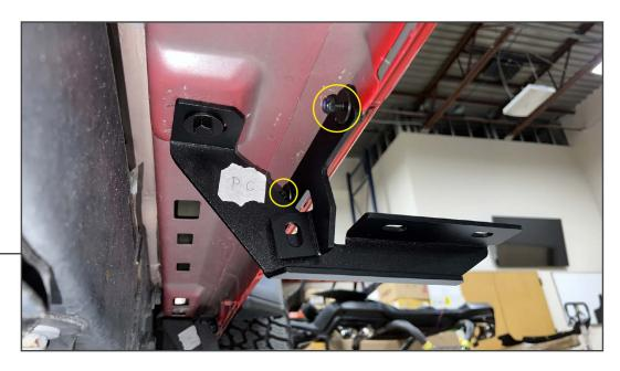
Loosely secure each appropriate rocker panel mounting bracket to the vehicle using (2) M6 x 25mm bolts, (4) M6 flat washers, and (2) M6 lock nuts through the vehicle pinch weld.
