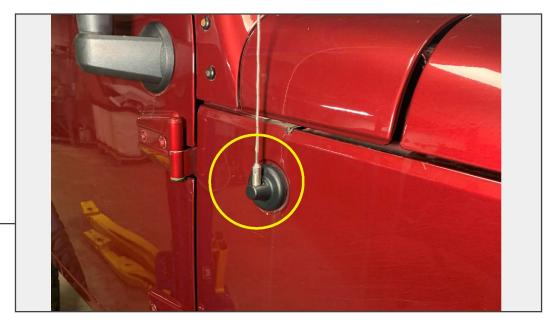
Clean vehicle. Remove vehicle antenna using an adjustable wrench.
